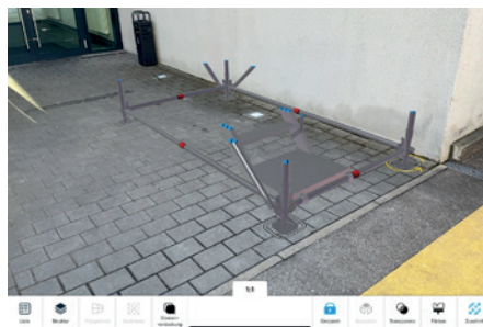
Augmented reality mode with cutting function (limit box) for visualising parts of the scaffolding structure
